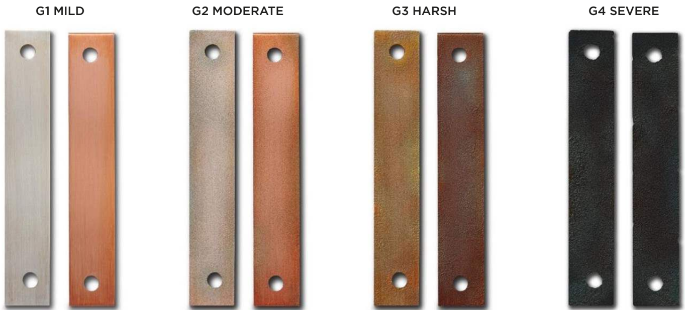
Above: Carboactiv Corrosion Coupons show the level of corrosive compounds in the air.
